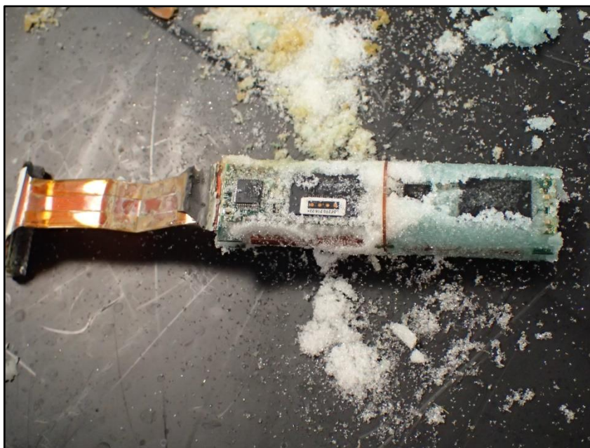
Photo No. 1: APMB from EI-ICR showing copper based insulation staining of glass beads
