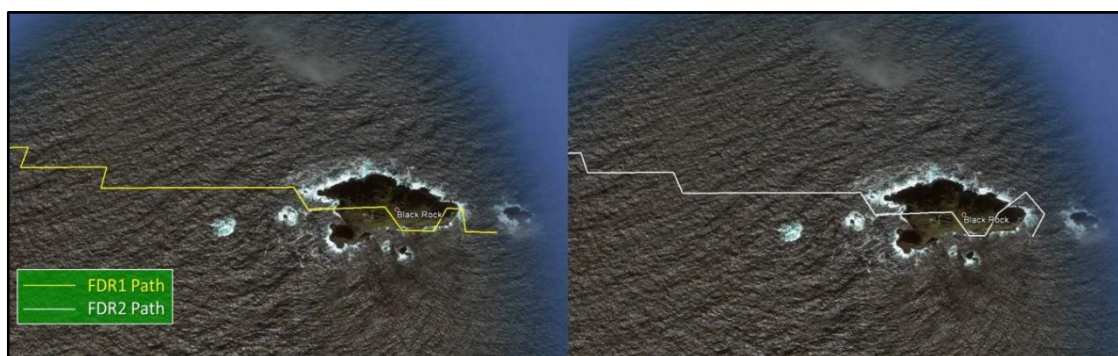
Figure No. 2: Position data from FDR1 and FDR2 showing the flight path of EI-ICR
